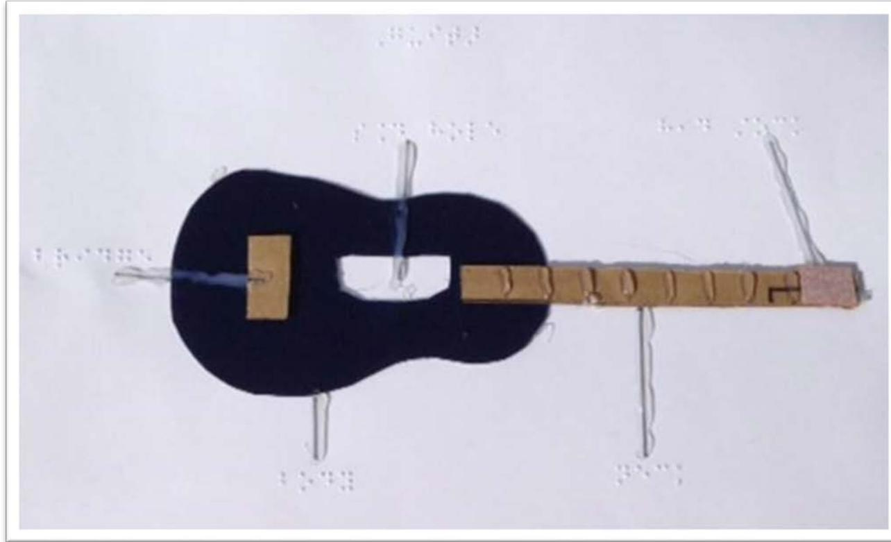
The lead lines with hot glue were “too strong” for the tactile reader and there was not an 1/8 inch between lead lines and other elements.
