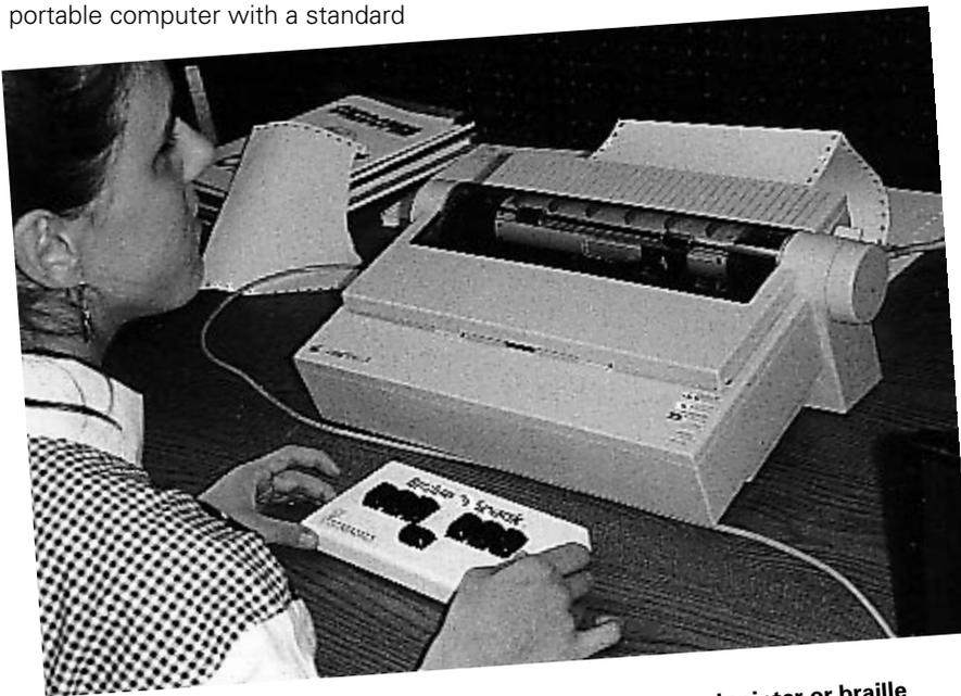
*A Braille 'n Speak can be connected directly to a conventional printer or braille embosser. Files created on a Braille 'n Speak can also be easily transferred to a desktop computer.*
