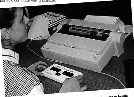
A Braille 'n Speak can be connected directly to a conventional printer or braille embosser. Files created on a Braille 'n Speak can also be easily transfered to a desktop computer.
